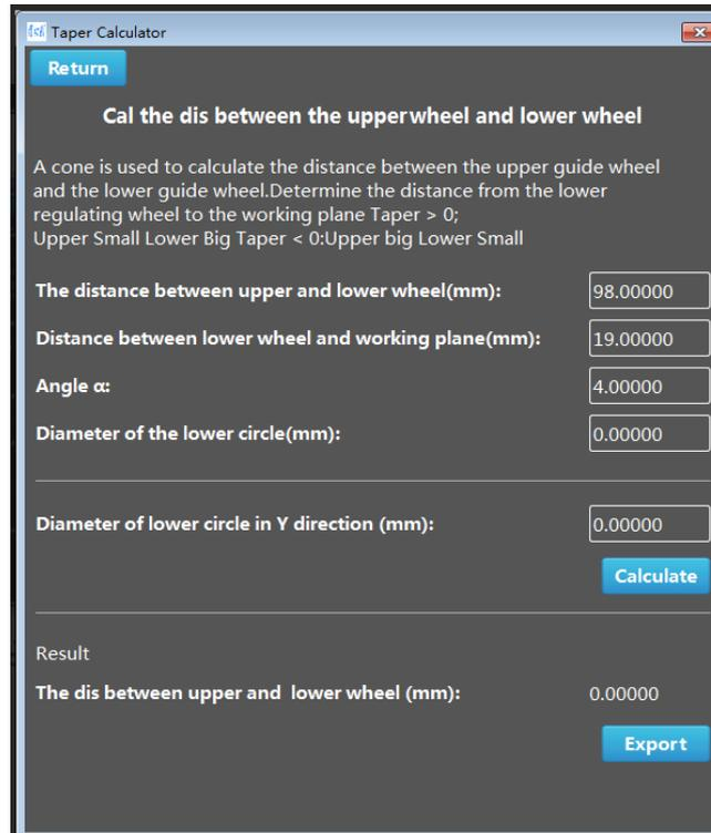
image 4-7-2 calculate the distance between upper and lower wire guide
