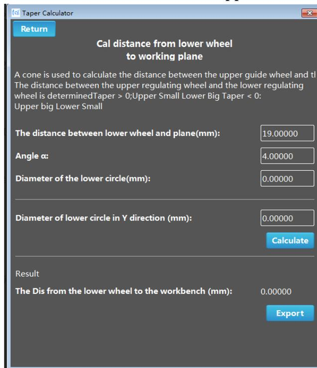
image 4-7-3 calculate the distance from lower wheel to working plane
